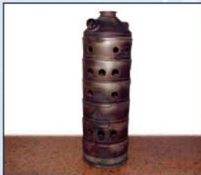
Combustion Liner, before
